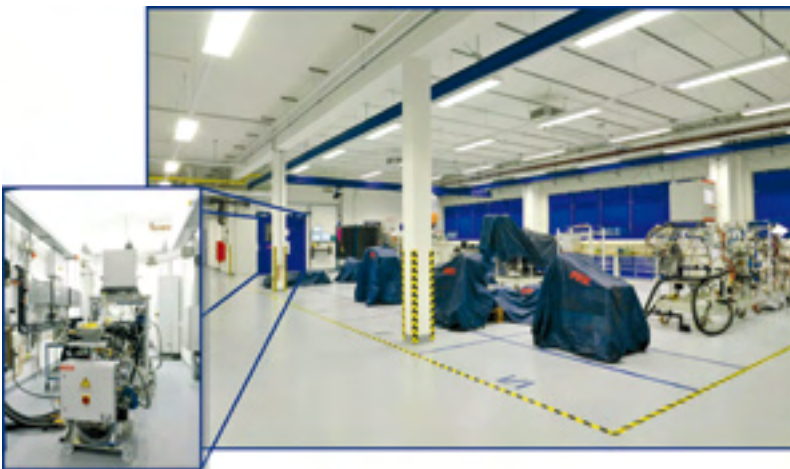
Figure 5: Openly arranged engine preparation area with test cell for pre testing
