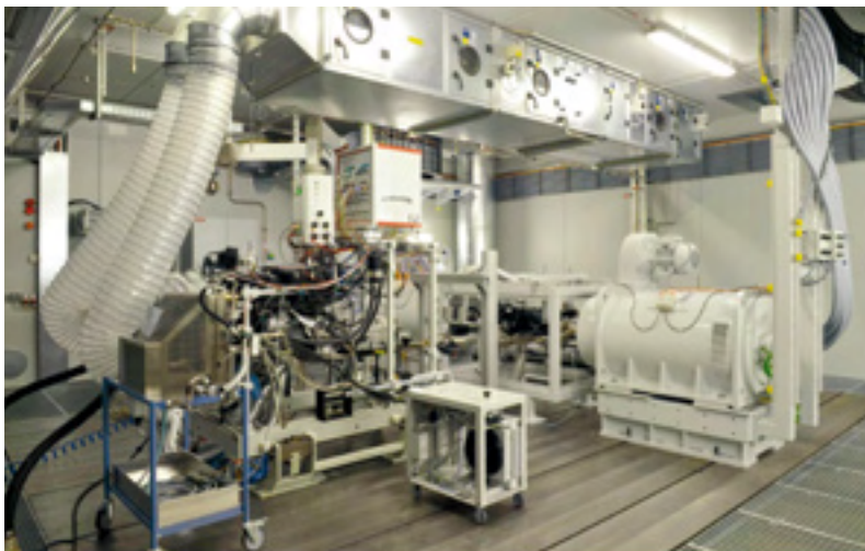
Figure 13: Power train test cell – here with transmission system components of a two-wheel-drive vehicle
