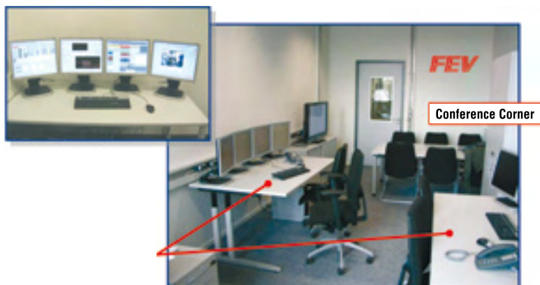
Figure 16: Virtual control center at a FEV customer's site respectively at FEV in Aachen to follow up test runs after electronic granting of access
